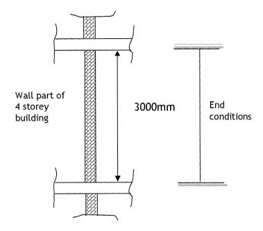
Determine the fire resistance period of a single leaf 102,5 mm brickwork wall constructed in Group 1 standard format clay masonry brick units assembled in an M4 general purpose mortar. The masonry unit gross dry density is 1600 kg/m<sup>3</sup>. The design vertical load is 180 kN/m and the design resistance is 207 kN/m.
